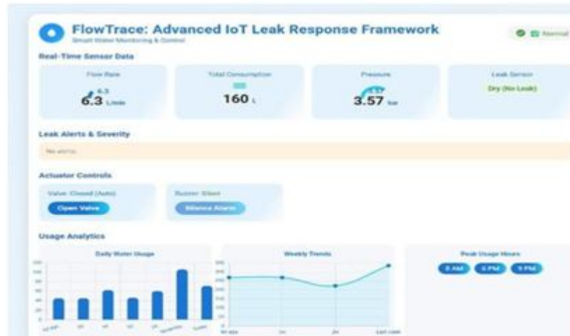
Fig.4. Cloud Dash board for real-time leak monitoring and analytics
