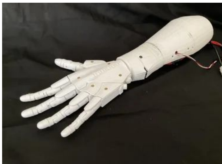
Fig 2. depicts a 3-d printed prosthetic arm which shows the rear forearm along with wrist joints, palm and fingers( each with respective protectors).
