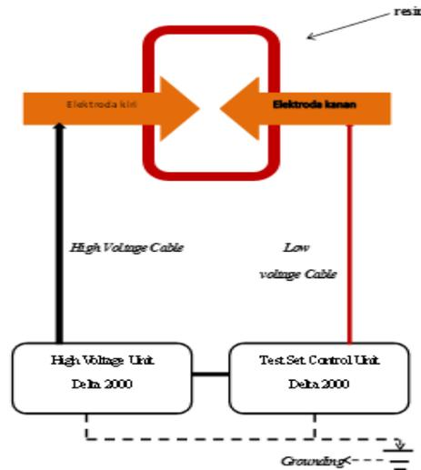
Figure 4 Diagram Testing Tangent Delta Transformer Oil
