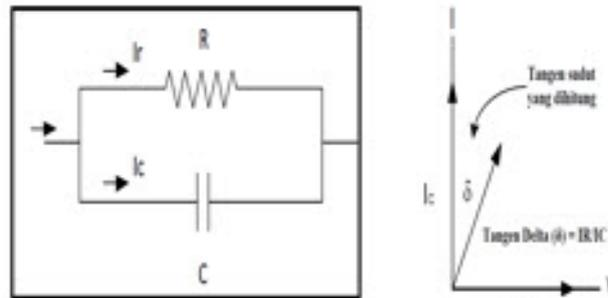
Figure 1 Equivalent circuit isolation and testing current phasor diagrams tangent delta
