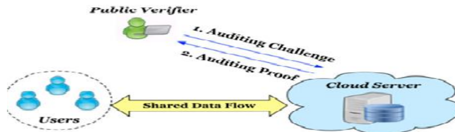
Fig.1 System model includes A cloud server, group of users and TPA(Public Verifier)
