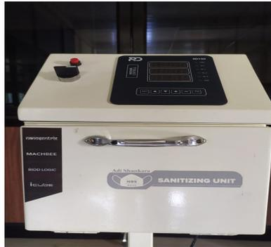
Fig. 5 Proposed UV chamber for N95 mask
