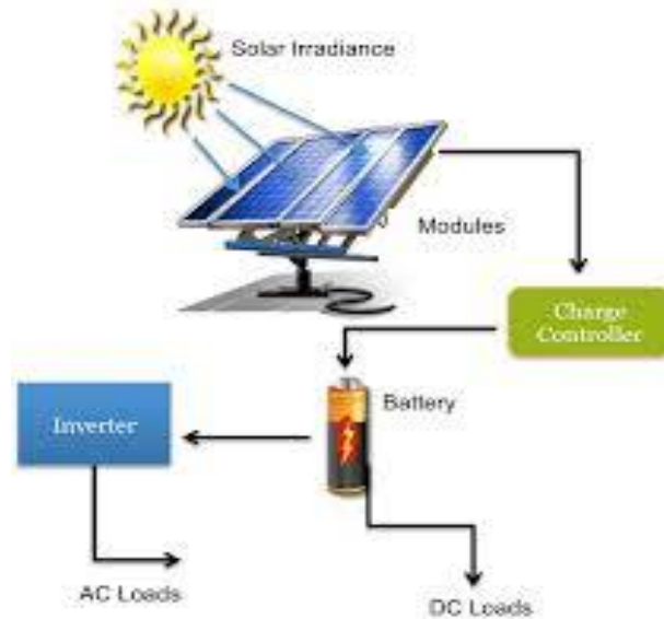
Fig. 1. How solar panel system works [6]
