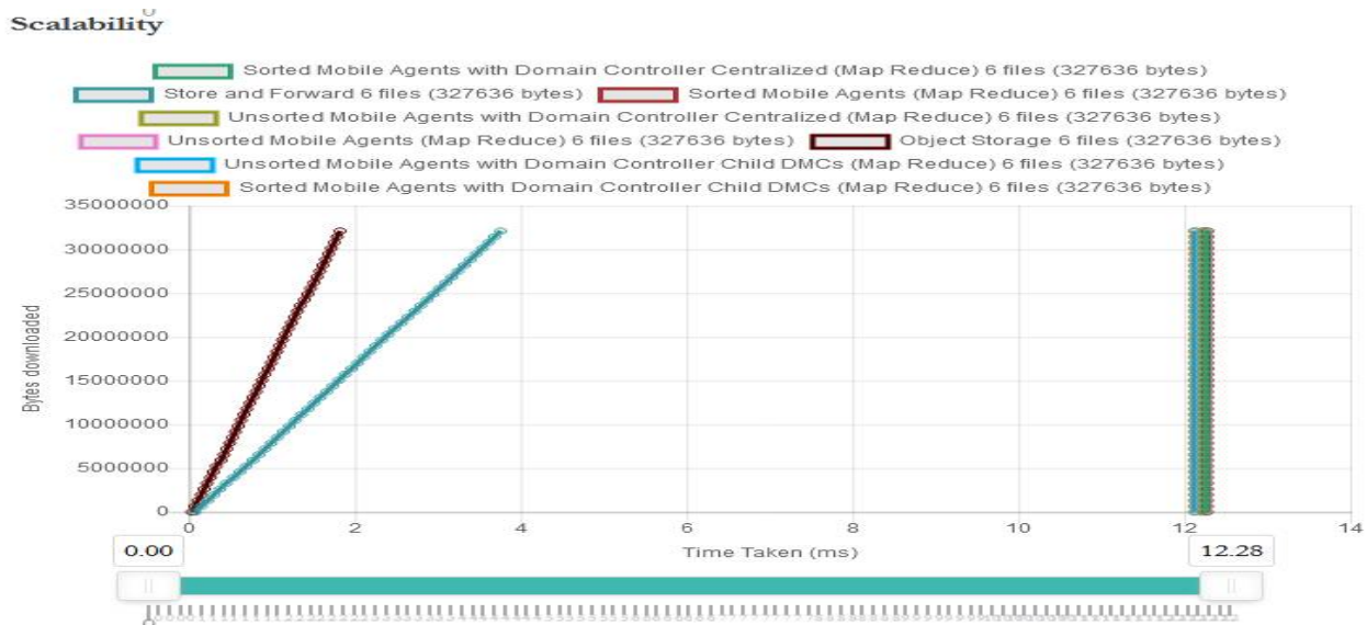
Fig 1.12: Scalability of 100 client requests for OSD, SAF and Sorted, Unsorted Mobile Agents with Map-reduce distributed over three different SAN containers.
